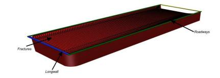
Figure 3: Model interpretation of mining induced floor fractures.
